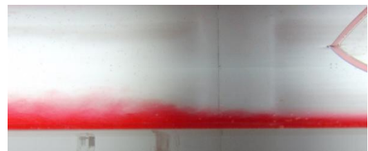
Fig. 5.4: Turbulent mixing of salt water from the hose, which slowly sets on the tank bottom with tap water above.
